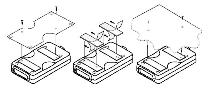
1. Installation with the installation plate supplied with the radio modem. The installation plate is fastened to the backside of the radio modem.
