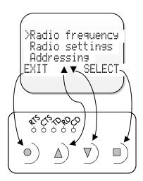
Pressing DOWN ( $\blacktriangledown$ ) button the cursor moves downwards. Depending on the sub-menu, the button also scrolls the digits of numerical values when changing some settings.
